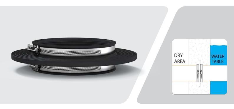
The Fernco Puddle Flange is designed to prevent leaks around pipelines penetrating poured concrete walls, floors, shafts, tanks, pools, manholes, and structures. The flexible gasket is installed during construction on the outside diameter of the pipe where a water tight seal is required. The unique flexible design bonds to concrete and compresses during the pour and curing process providing a leak proof seal against water and gas.
